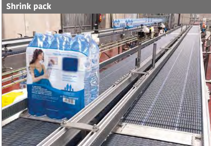
LBP: basically for accumulation GT: basically for inclines/declines and stop-divider applications
