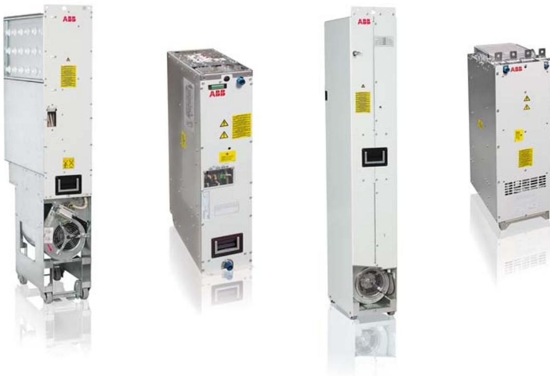
ABB's multidrive modules are designed to be installed in cabinets that feature a common DC bus. They are available as inverter modules, supply modules and braking choppers and resistors, and cover a wide range of applications. These modules contain all the drive technology and different types of supply units that convert the AC supply from the mains into a DC supply for the inverter modules. ABB provides full engineering support for designing cabinets.
